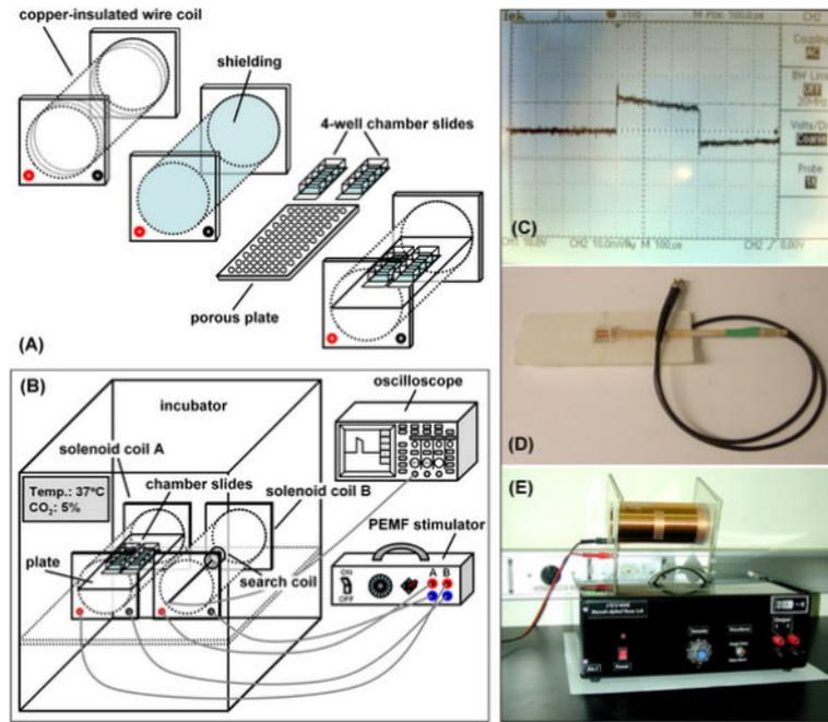
**Figure 1.** The PEMF stimulation system: (A) solenoid coils with porous plastic board placed horizontally in the center; (B) control units for regulating and monitoring the signals derived from solenoids placed inside an incubator; (C) induced electric field with single quasi-rectangular pulse; (D) a search coil for detecting induced electric fields; and (E) PEMF stimulator and solenoid coil.
